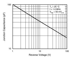
Fig. 5 - Typical Junction Capacitance
