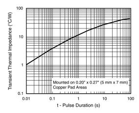
Fig. 6 - Typical Transient Thermal Impedance
