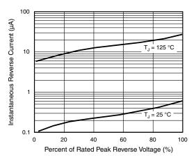
Fig. 4 - Typical Reverse Characteristics
