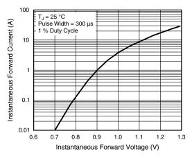
Fig. 3 - Typical Instantaneous Forward Characteristics
