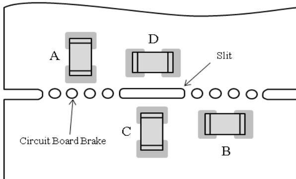
Stress strength according to the mounting position:
